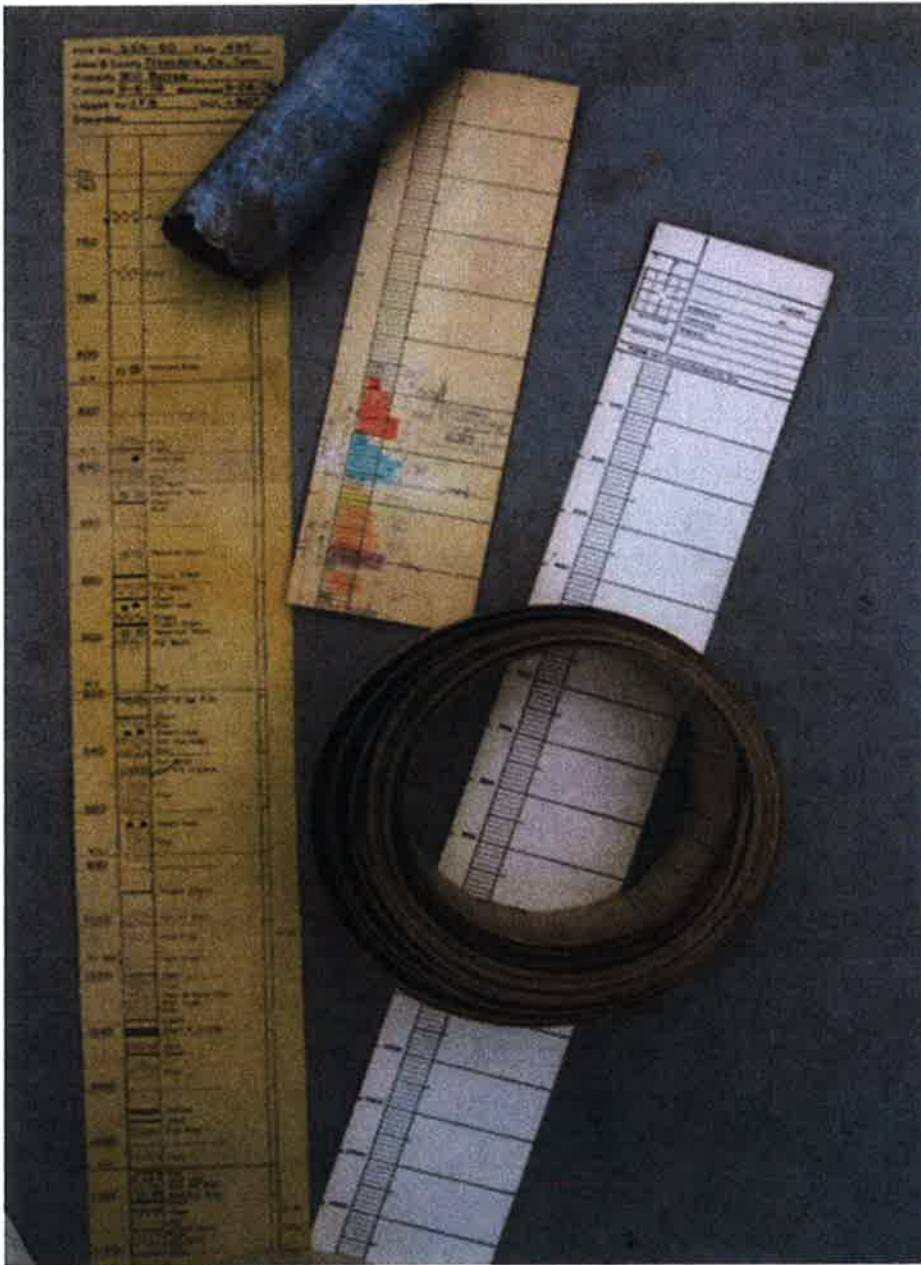
Figure 1. Photograph showing examples of strip logs. The log on the left exhibits graphic representations of the lithologies and features in the lithology column; feature descriptions are written out to the right. The short log in the center shows the lithologies with color, with sedimentary features shown graphically to the right. A strip log template and a roll of logs are shown on the right.
